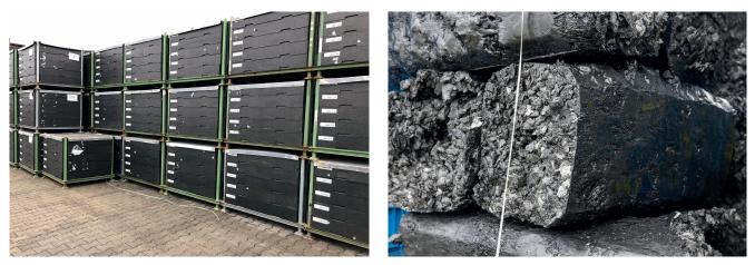
Fig. 2. Decommissioned load trays are collected, compacted, and then granulated (© JSP)
