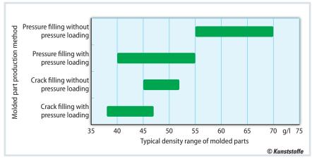
**Fig. 4.** Arpro 5134 RE can be processed using the crack filling or pressure filling method, with or without pressure loading (source: JSP)
