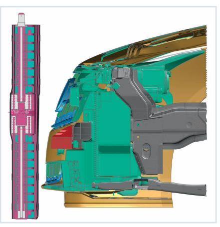
**Fig. 5.** Finite elements analysis (FEA) with the LS-Dyna software: safety-relevant areas in the automobile, like the pedestrian protection here, are tested via simulation. The area shown red in the simulation consists of EPP and absorbs some of the energy in case of a collision, e.g. with a pedestrian's leg (© JSP)
