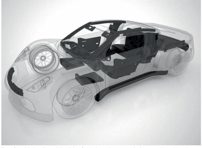
The use of expanded polypropylene in vehicles, including safety-critical areas such as passenger and pedestrian protection is vastly increasing (© JSP)
