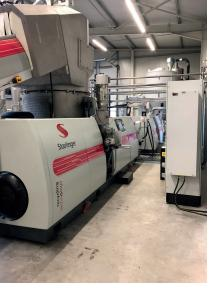
**Fig. 3.** At the Eschwege (Hesse) site, the collected load trays are processed to EPP granulate and subsequently examined for key properties in the laboratory (© GID)
