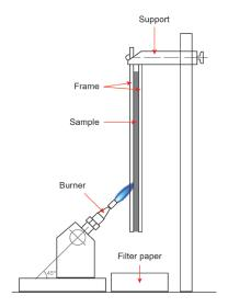
For classes E and F, only the ignition test with a small flame is required. For classes A1, A2, B, C and D the test EN 13823 is required.
