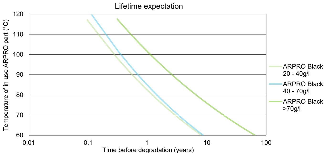
In order to use the curves, the minimum lifetime expected or the average working temperature has to be known. For instance, if the application requests a 10 years lifetime, then ARPRO can be used when the continuous working temperature is 60°C or below. If the application has to sustain a temperature profile (with various temperature cycles or differences between winter and summer), then the average temperature should be used as the reference to obtain the expected lifetime.
