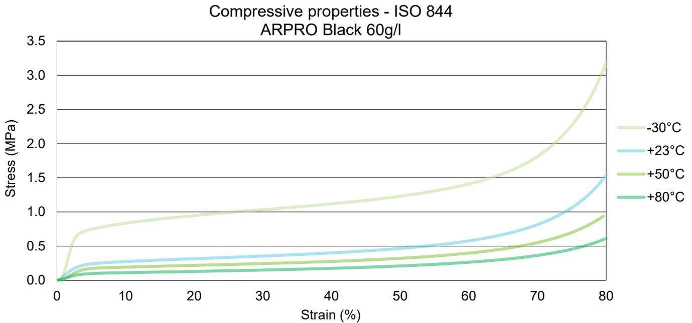
**Test result explanation:** When ARPRO is submitted to heat, the material will soften; some residual resistance will remain, even at high temperature. The general thermoplastic behaviour will remain steady whatever the temperature tested, even below the glass transition (around -10°C).
