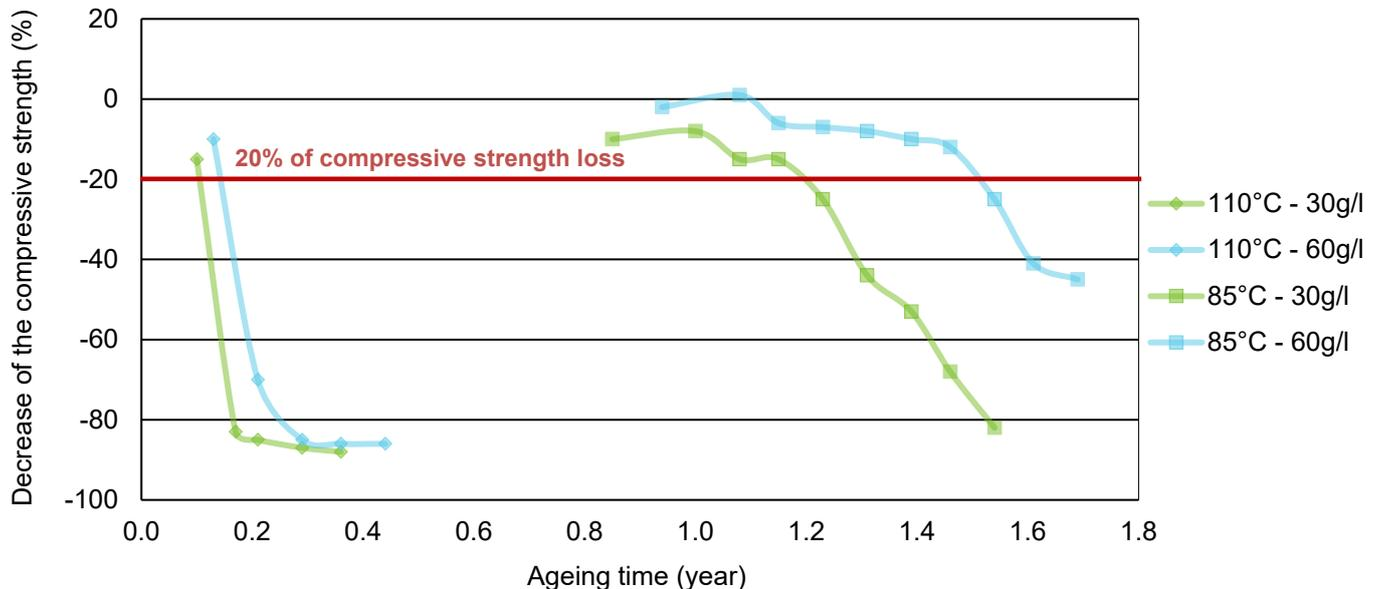
**Test results explanation:** At a constant temperature of 110°C, ARPRO at 30g/l and 60g/l will start degrading and losing performance after two months. At a constant temperature of 85°C, ARPRO at 30g/l will lose 20% of its initial compressive strength after 15 months. For ARPRO at 60g/l, this will occur after 18 months.
