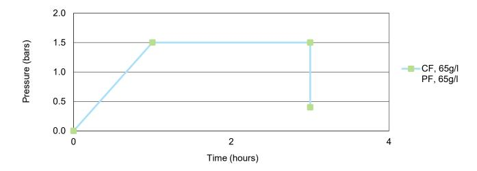
Pre-treatment cycles can be adapted according to moulding process, density and part geometry:
