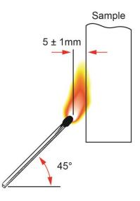
Test results: ARPRO 4135 FR at 60g/l, with a flame applied for 30 seconds:
