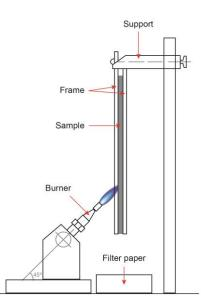
For classes E and F, only the ignition test with a small flame is required. For classes A1, A2, B, C and D the test EN 13823 is required.
