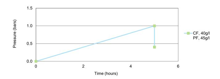
Recommended pre-treatment cycle with pressure tank environment and incoming compressed air both at 23°C: 5 hours up to 1 bar, decrease and maintain at 0.4 bar throughout production.
