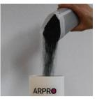
Introduce the material into the container at a 45° angle, transferring it carefully either from a receptacle or simply by hand\*\*\*. Avoid shock or forced compaction.
