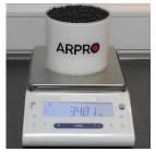
4. Weigh the full container and record the result with accuracy up to one decimal.
