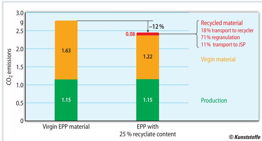
**Fig. 1.** Compared with virgin EPP from JSP, 1 kg of EPP with 25% recyclate content generates 12% less CO<sub>2</sub> emissions (source: JSP)
