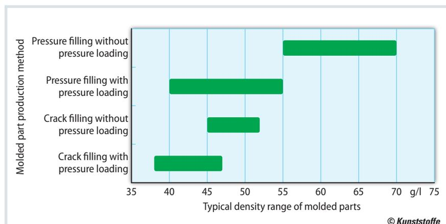
**Fig. 4.** Arpro 5134 RE can be processed using the crack filling or pressure filling method, with or without pressure loading (source: JSP)
