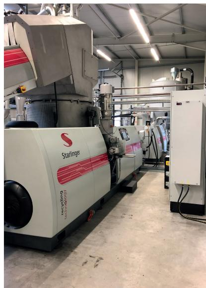
**Fig. 3.** At the Eschwege (Hesse) site, the collected load trays are processed to EPP granulate and subsequently examined for key properties in the laboratory (© GID)
