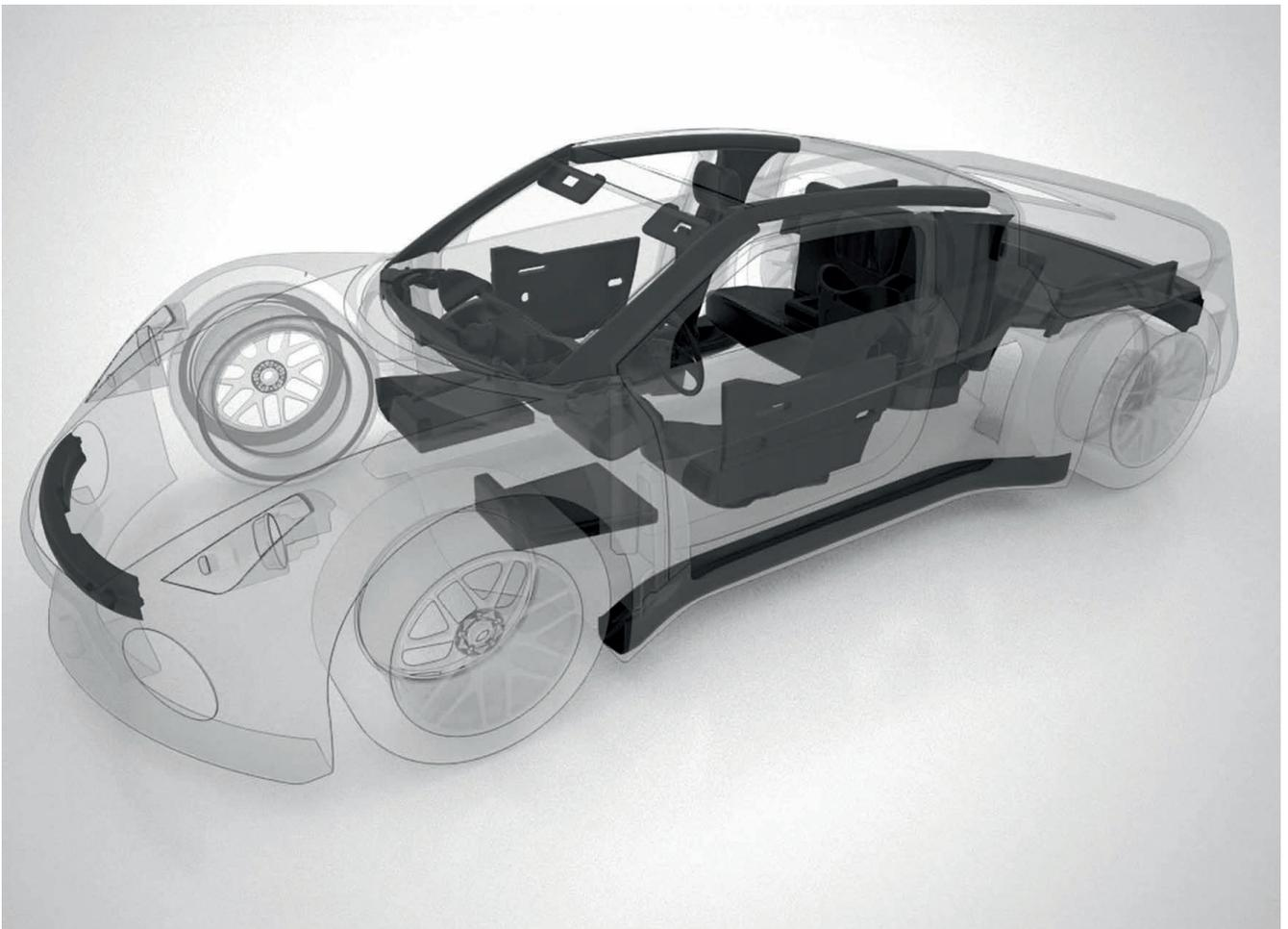
The use of expanded polypropylene in vehicles, including safety-critical areas such as passenger and pedestrian protection is vastly increasing (© JSP)
