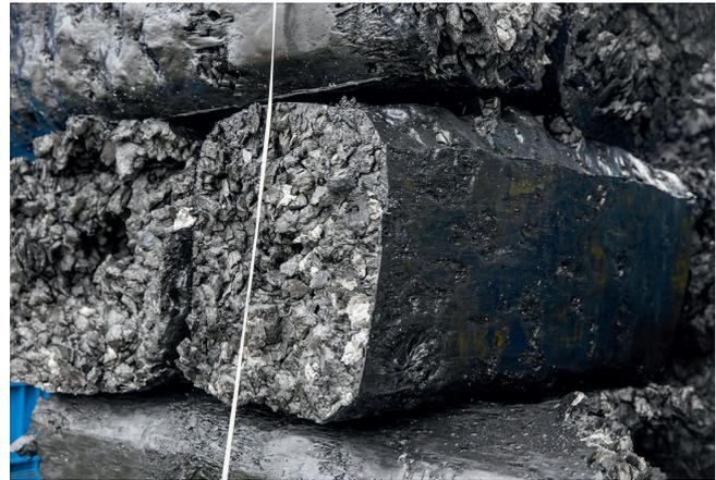
**Fig. 2.** Decommissioned load trays are collected, compacted, and then granulated (© JSP)
