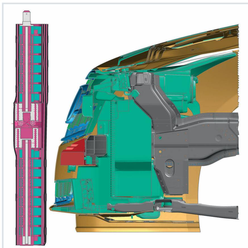
**Fig. 5.** Finite elements analysis (FEA) with the LS-Dyna software: safety-relevant areas in the automobile, like the pedestrian protection here, are tested via simulation. The area shown red in the simulation consists of EPP and absorbs some of the energy in case of a collision, e.g. with a pedestrian's leg (© JSP)
